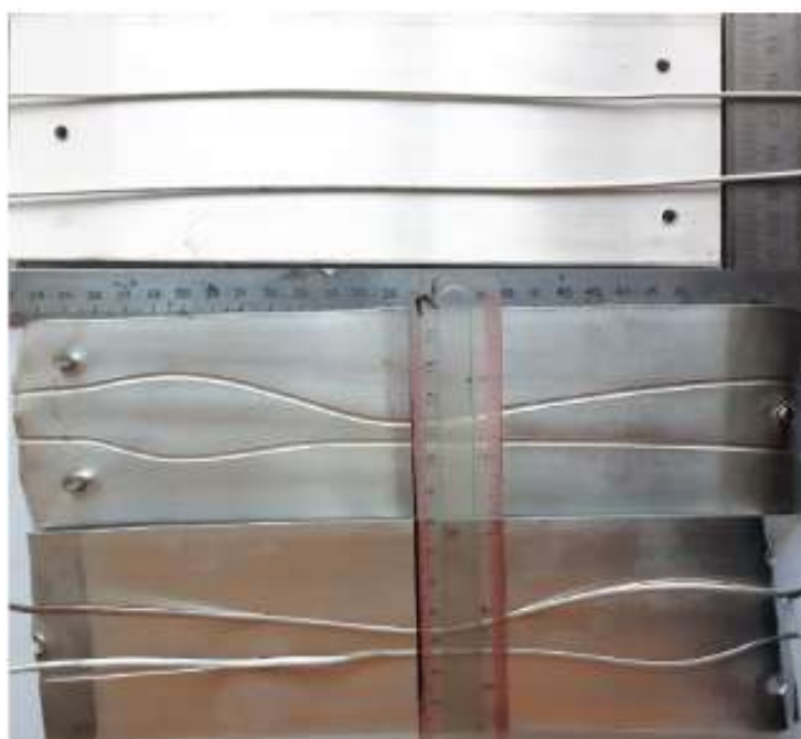
Figure 3 – Aluminum wire before and after rolling
