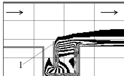
Figure 3 – Distribution of dust concentration, t = 15 : 1 – brattice
